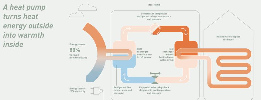
With Aquarea up to 80% of the heat energy required is taken from the ambient air. Aquarea captures heat energy from the ambient air and transfers it to heat the water needed to warm your home for domestic hot water and even to cool the house if wished.
